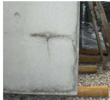
Day 3-Crystals begin to grow filling the cracks
