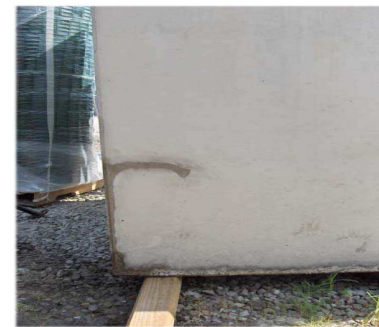
Day 1 Leaks appear as the tank is filled
