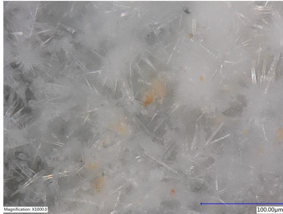
Figure 3: Crystal growth in cracked concrete (Magnification x1000)
